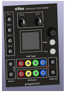
Before installing the front panel check that you have removed the protective covering from the OLED display. Check the red LED is still in the correct position and protrudes through the front panel hole. There should be a small amount of play around the push buttons, check that they are loose and easy to press.
