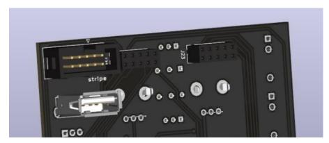
Insert the 16 pin Eurorack header into the back of the PCB. The key-slot must be at the **outer edge** of the PCB, turn the PCB over and solder the connector in place. As before, solder one pin and check that the connected is flush with the PCB before soldering the remaining pins.
