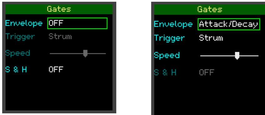
The Gates page configures how and when the internal envelope generator or sample-and-hold (S&H) are triggered. The **Envelope** parameter has three values: **OFF** which disables the envelope generator, **Attack/Decay** to configure the envelope generator as an attack/decay envelope, and **ADSR** to configure the internal envelope generator as an attack/decay/sustain/release envelope.
