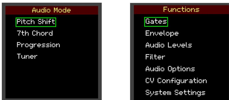
Selecting **System Settings** on the Functions menu page brings up another menu page that lists infrequently used functions such as changing the display settings, recalibrating the VPO inputs or viewing the firmware version.
