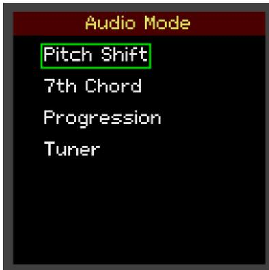
Pitch Shift mode provides independent control of the output pitch of the four voices with optional quantization to a selected scale.
