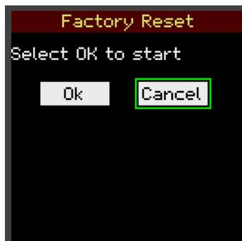
The Factory Reset page is used to restore all configurations settings to their original values. This includes resetting all the CV assignments, setting the CV and VPO calibration offsets to 0.0 and scale factors to 1.0. This is probably something most users will rarely need to do. To do a factory reset, open the Factory Reset page and use the rotary encoder to select and click on the **Ok** button.
