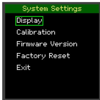
Most changes to settings made via the user interface, including the most recent audio mode, are stored to flash memory, and restored when the module is next powered on. Selecting **Factory Reset** from the System Settings menu page sets all configurable settings to their original defaults.
