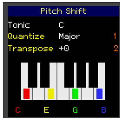
In the right-hand example both the **Quantize** and **Transpose** parameters have been configured for CV control. Assigned parameter names appear in yellow and the numbers at the right-hand side of the display show which CV input is controlling that parameter. CV assignments are set from the **CV Configuration** page and the selected assignments are saved to flash memory.
